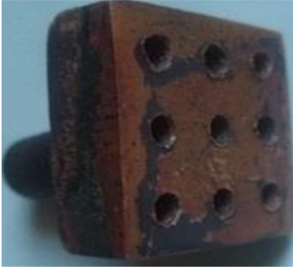
Fig. 4.3. Cu tool with array of holes
