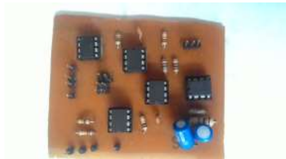
Figure 19 : Final Circuit of ECG DAQ (Front)
