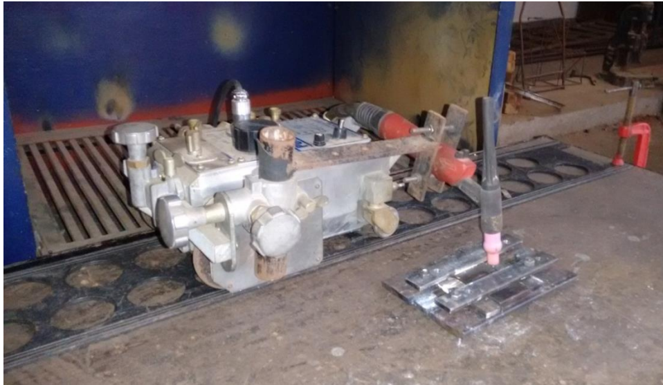
Fig. 5 Movable vehicle holding the welding torch
