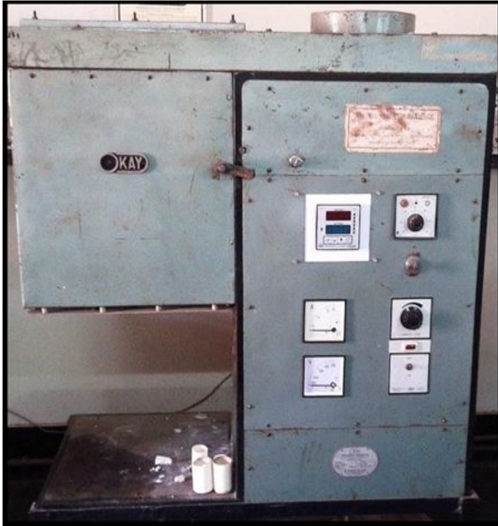
Fig.3.5. Rising Hearth Furnace
