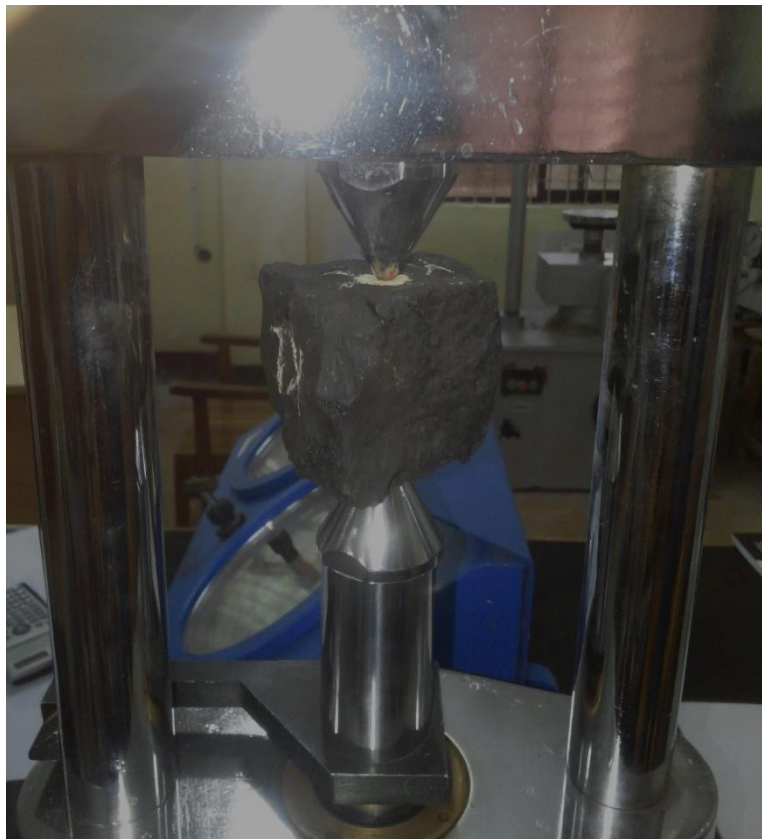
Figure 4.2:- Point Load Testing Machine after loading of sample
