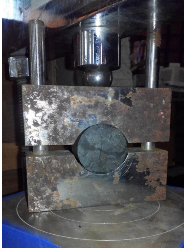
Figure 4.4:- Brazilian Tensile Strength Test
