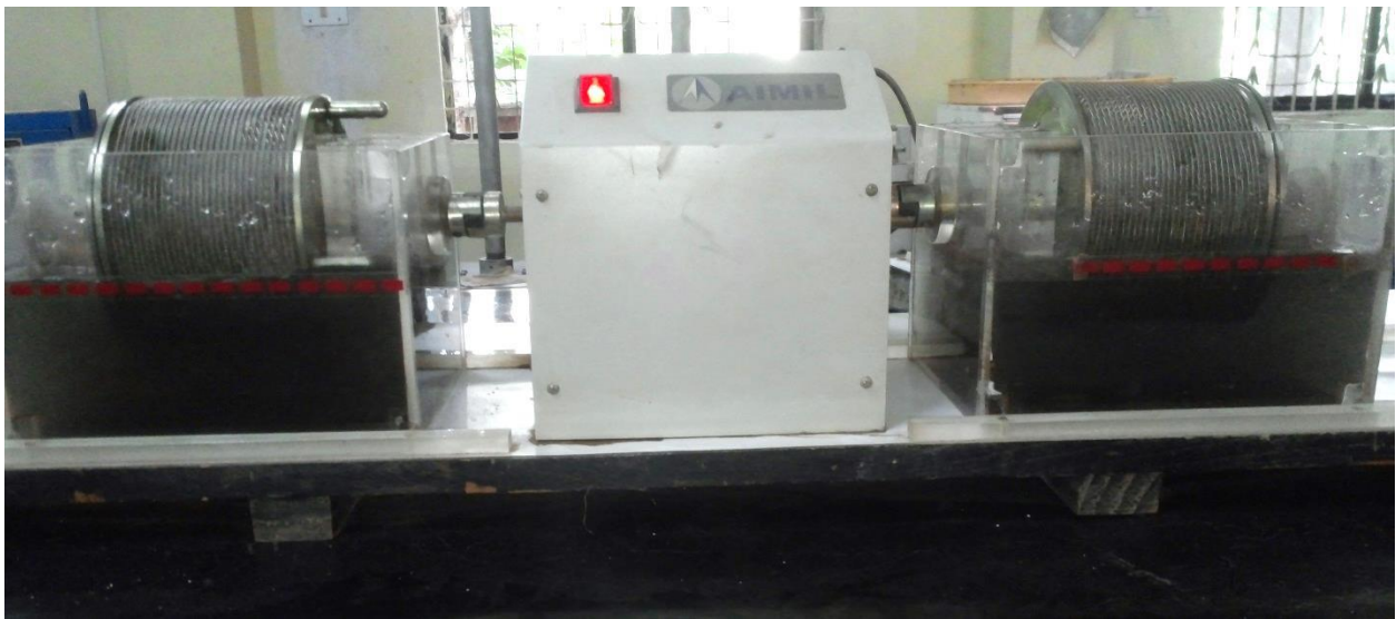
Fig 4.6:- Slake durability Test coal samples
