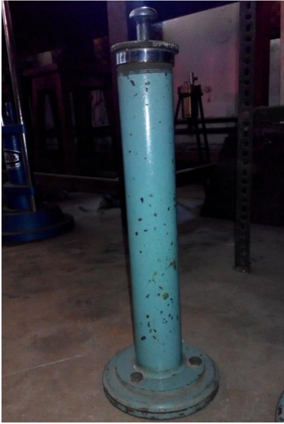
Figure 4.7:- Impact Strength Unit (Cylinder with plunger) and Sample of coal
