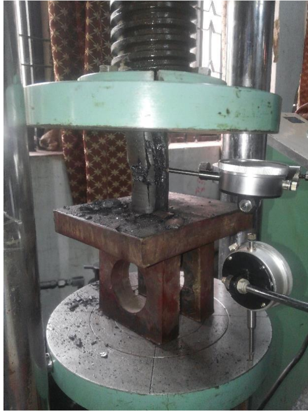
Figure 4.3:- Unconfined Compressive Strength test after failure of coal specimen
