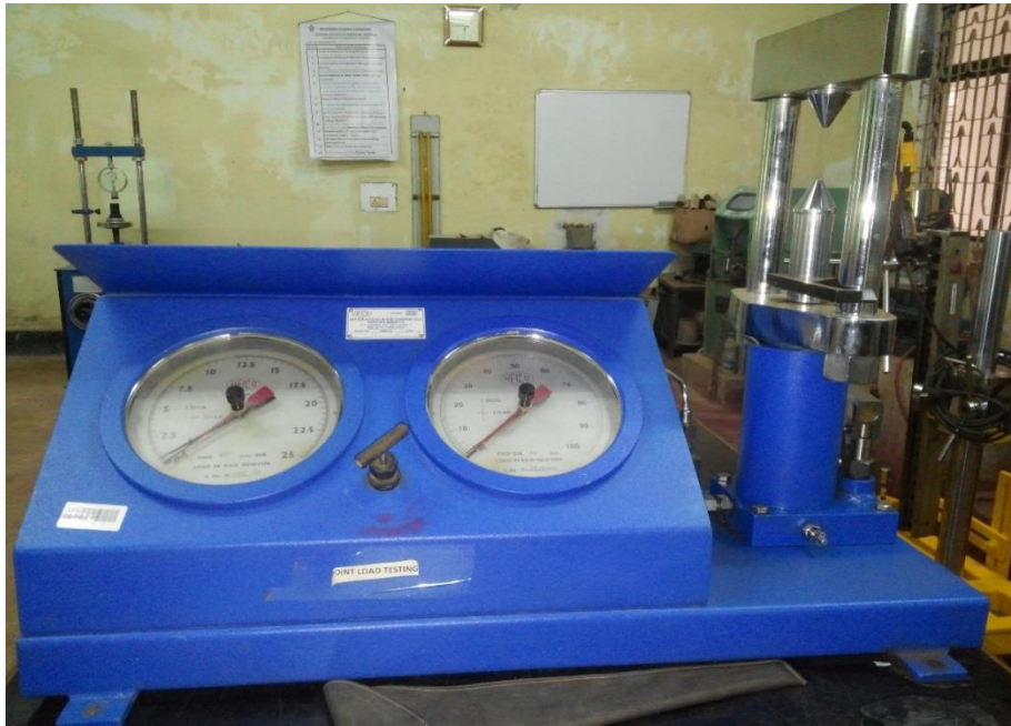
Figure 4.1:- Point Load Testing Machine before loading of sample
