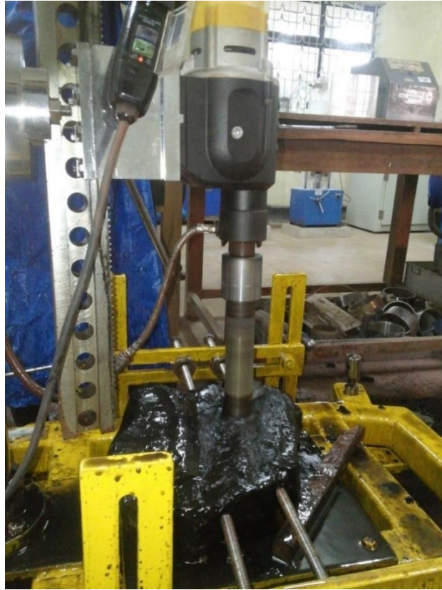
Figure 3.4:- Coring of Coal Block using Drilling Machine
