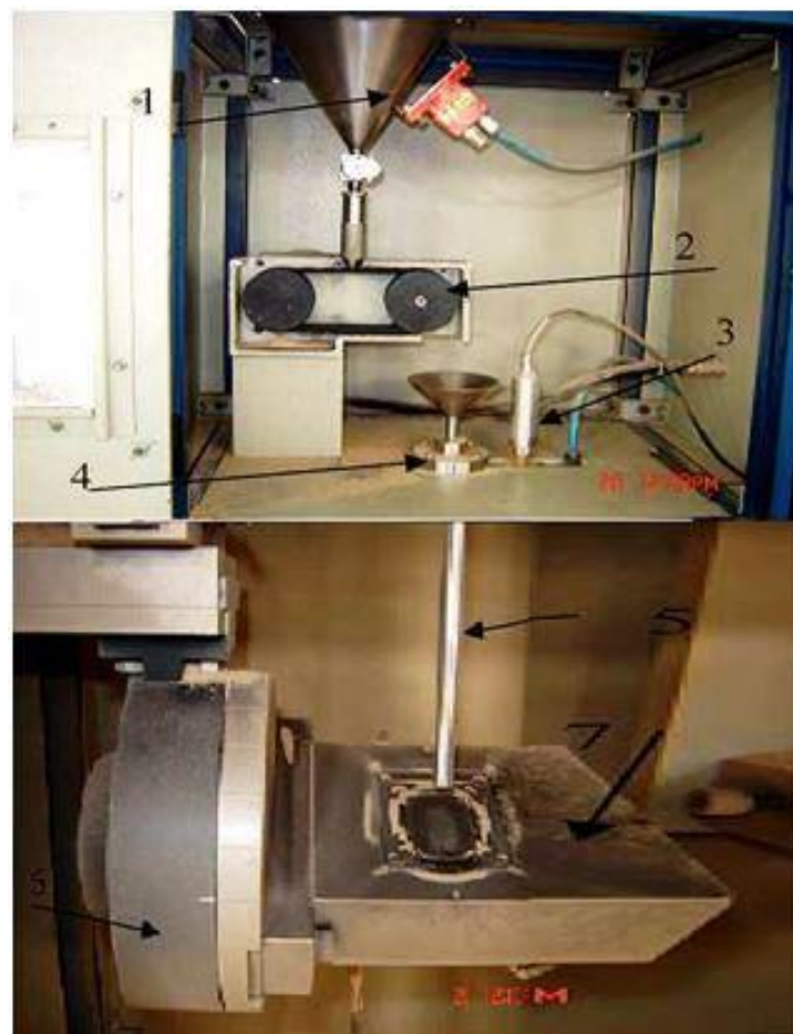
Figure-4.1 Details of erosion test rig. (1) Sand hopper, (2) Conveyor belt system for sand flow, (3) Pressure transducer, (4) Particle-air mixing chamber, (5) Nozzle, (6) X- Y and h axes assembly, (7) Sample holder
