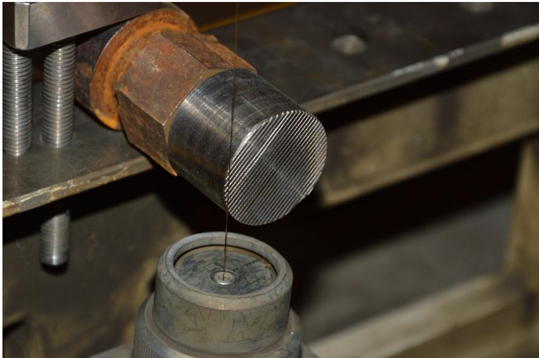
Fig. 3.4 Wire EDM cutting (status: M/C OFF)
