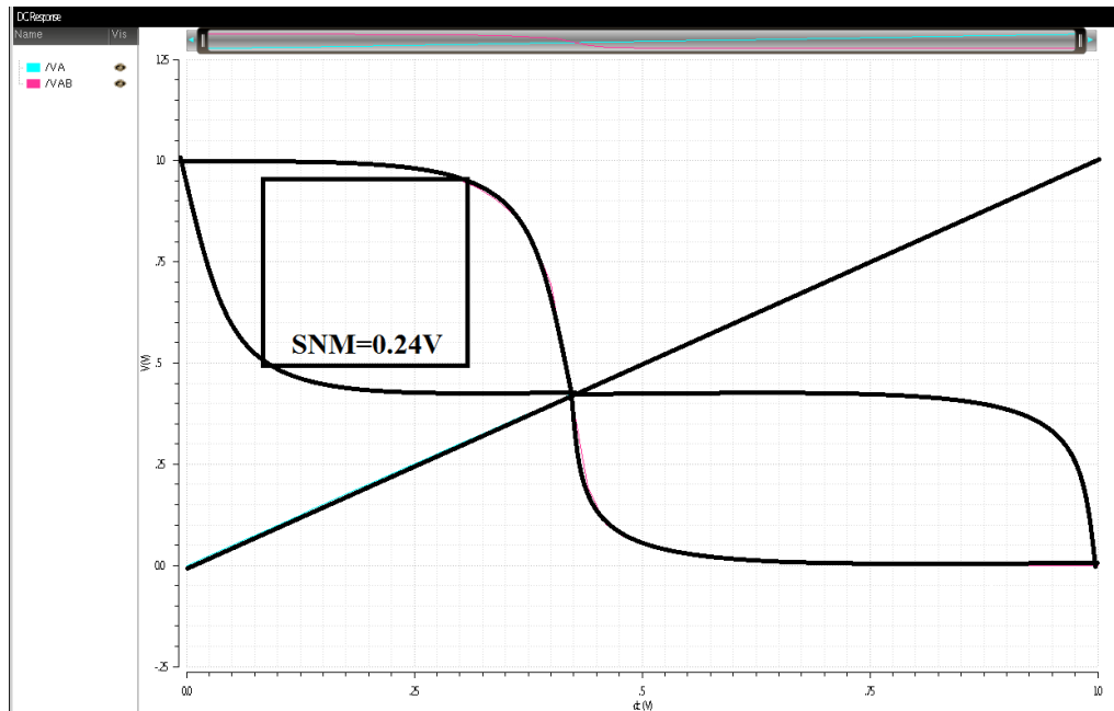
Fig.4.8 static noise margin representation of 6T-cell
