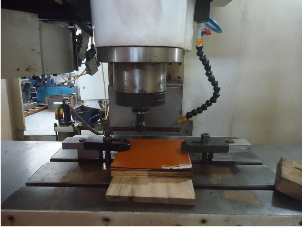
Fig. 3. Experimental setup of micro-drilling of PCB.
