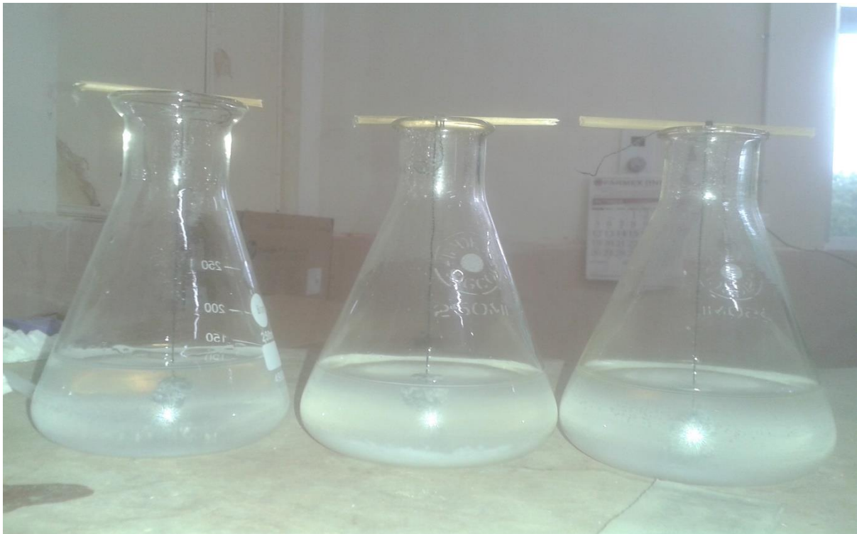
Figure 3.6: Specimens hanged in the beaker containing salt solution.
