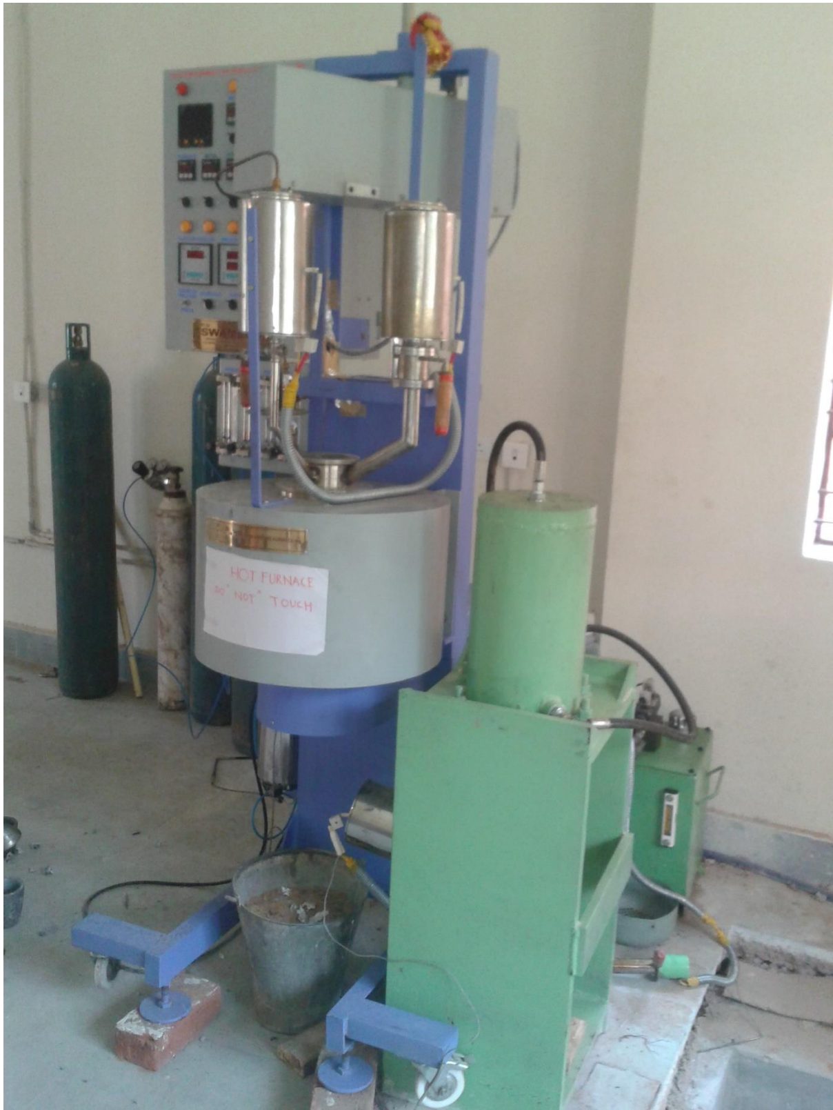
Figure 3.1: Bottom pouring type furnace used for melting
