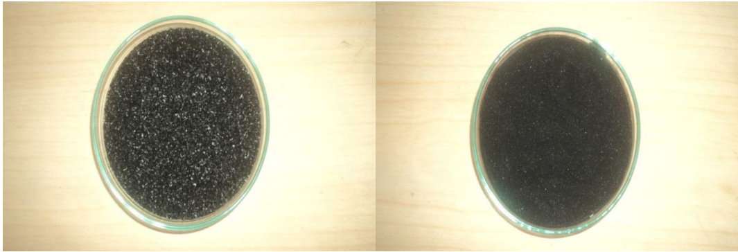
Fig 3.3 Granular activated carbon
