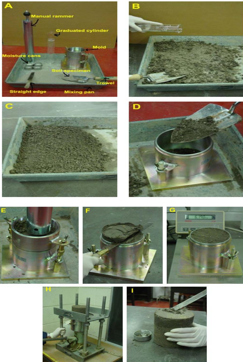
Figure 20: Steps involve in Procter Hammer Test
