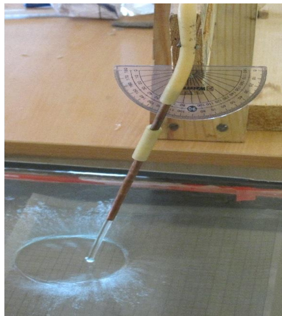
Fig.5.5 Non- Circular Hydraulic jump due to oblique jet impingement.
