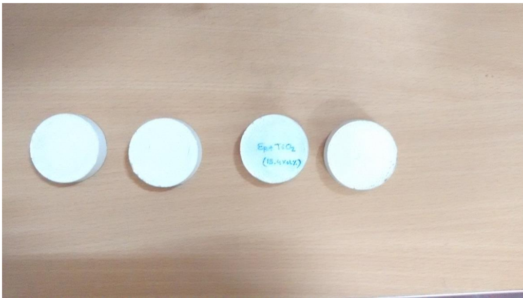
Figure 3.6 Fabricated composite for filler volume fraction of 6.7%, 13.4%, 26.8% and 40.2%
