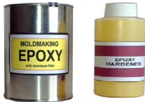
Figure 3.3 Epoxy resin and its corresponding hardener
