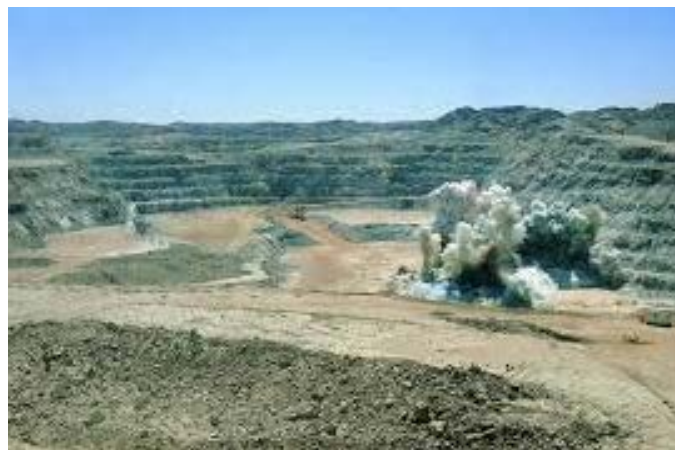
Figure 3.1 Particulate generation from Blasting Operation
