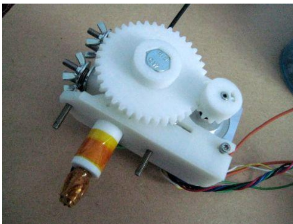
Fig-25: Wade's geared extruder
