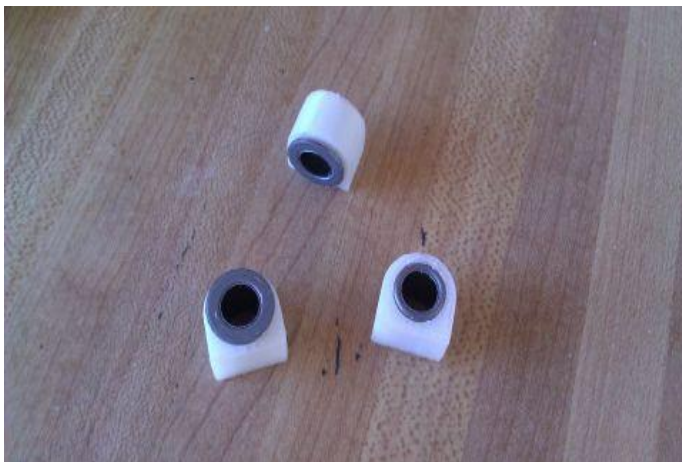
Fig-20: Brass Bushing inserted in printed parts
