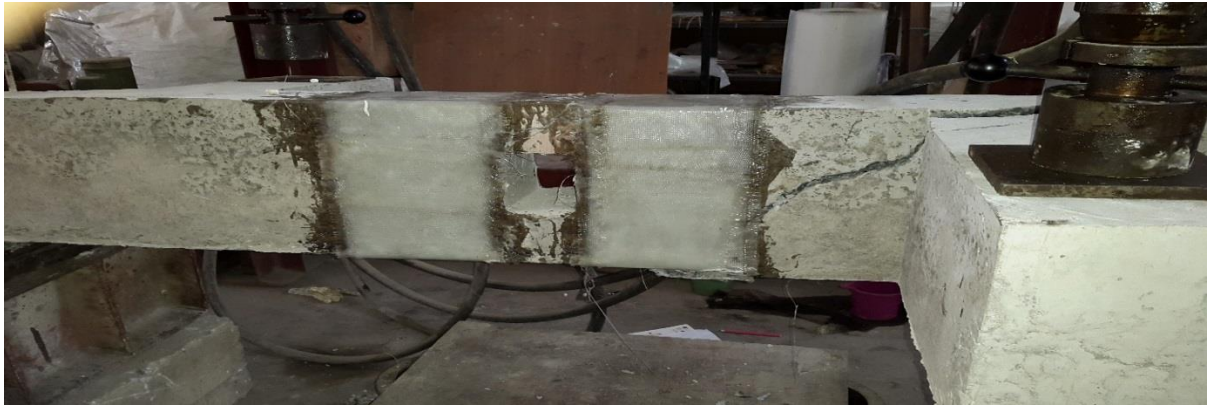
Fig 4.11(b) Crack pattern in BSRO4
