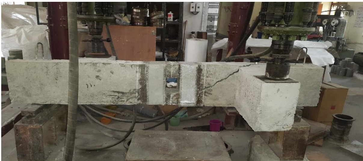
Fig 4.9(b) Crack pattern in BSRO2
