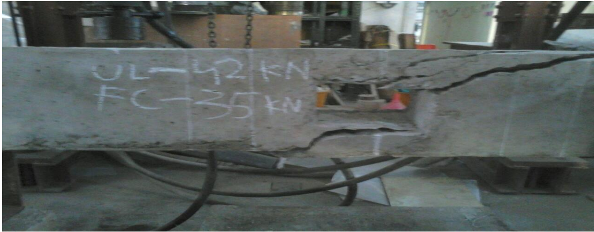
Fig 4.2(b) Crack pattern in BRO
