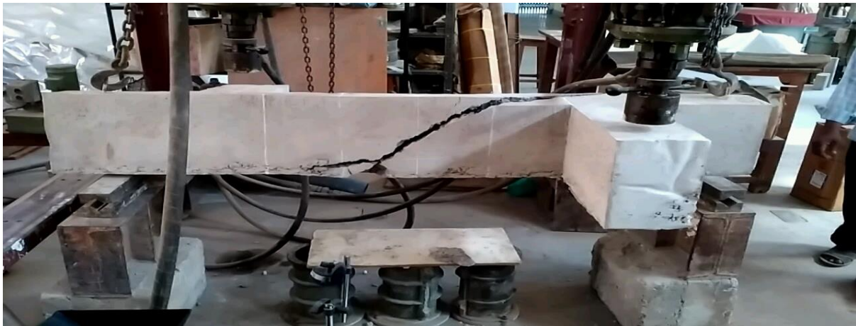
Fig 4.1 Crack pattern in CB
