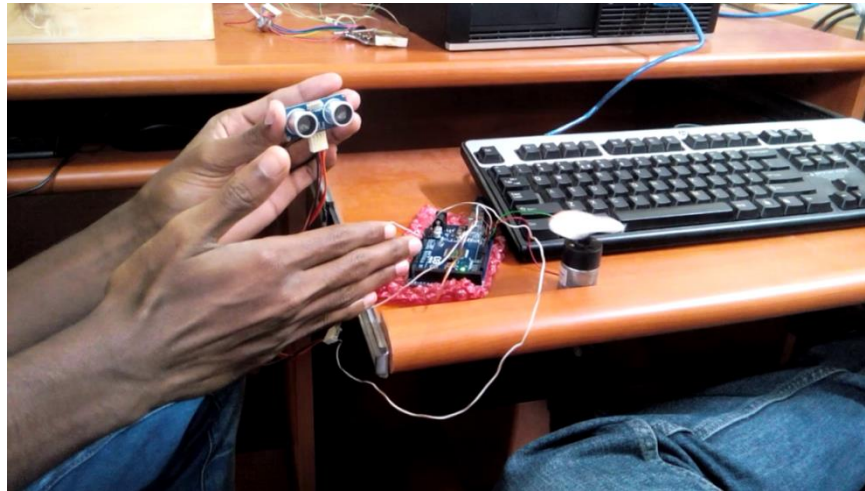
Figure3.8 Interfacing of the DC motor with Ultrasonic
