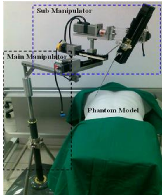
Figure 1.1: Transcutaneous Robot-assisted Ablation-device Insertion Navigation System [1]
