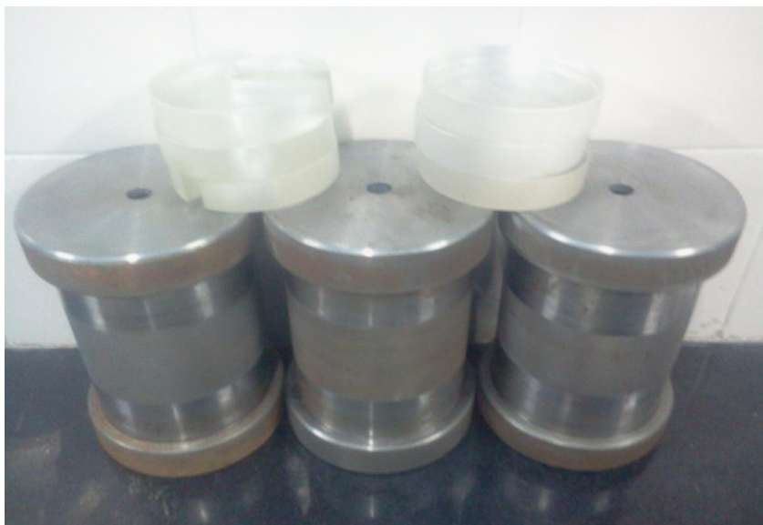
Fig. 4.6 Photographic view of Mild steel moulds
