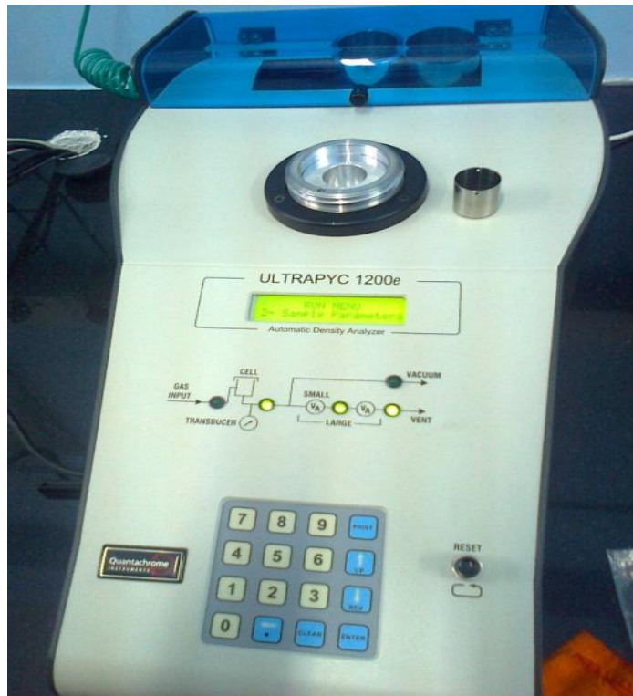
Fig. 4.1 Photographic view of helium gas pycnometer used for determining specific gravity of samples
