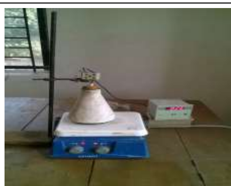
Figure 3.5: Actual diagram of experimental setup for higher temperature (Magnetic stirrer)
