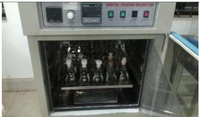
Figure 3.3: Orbital shaker arrangement
