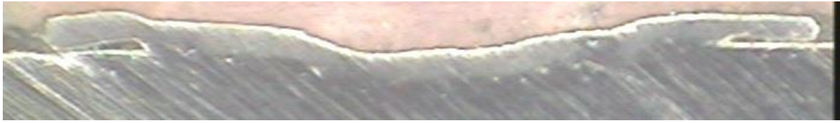
Fig .6: The magnified microscopic image of the cross section of the TIG clad AISI 304 stainless steel processed with 40 amp and scan speed of 5.3 mm/s
