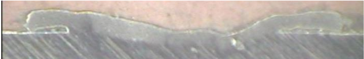
Fig .7: The magnified microscopic image of the cross section of the TIG clad AISI 304 stainless steel processed with 40 amp and scan speed of 6.5 mm/s
