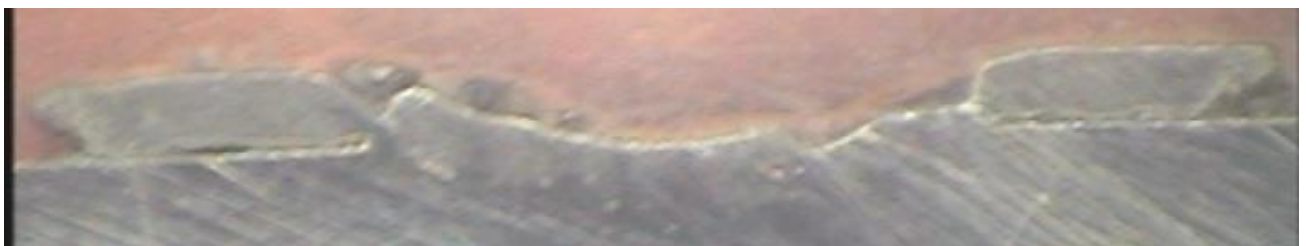
Fig .10: The magnified microscopic image of the cross section of the TIG clad AISI 304 stainless steel processed with 60 amp and scan speed of 5.3 mm/s
