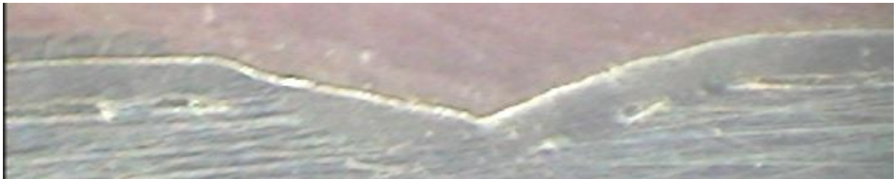
Fig .8: The magnified microscopic image of the cross section of the TIG clad AISI 304 stainless steel processed with 50 amp and scan speed of 5.3 mm/s
