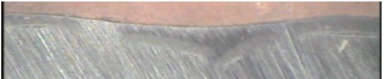
Fig .12: The magnified microscopic image of the cross section of the TIG clad AISI 304 stainless steel processed with 80 amp and scan speed of 5.3 mm/s
