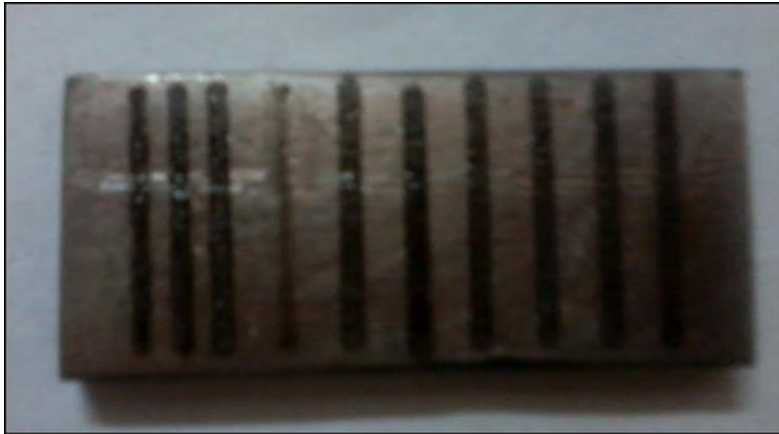
Fig .3: TIG cladding on AISI 304 stainless steel with different parameter combination
