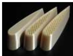
Fig 6. Different fills schematically
