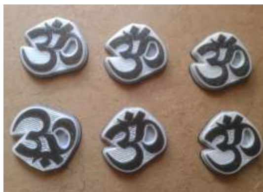
FIG 7: OM printed using various fill types
