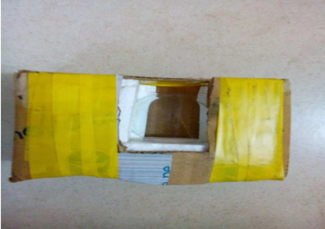
Figure 7(a): Positioning of the finger if no device for keeping finger is made (b): Cardboard made where the finger is inserted inside the hole seen (c): Bottom view of the cardboard with lens attached on which the finger is to be placed
