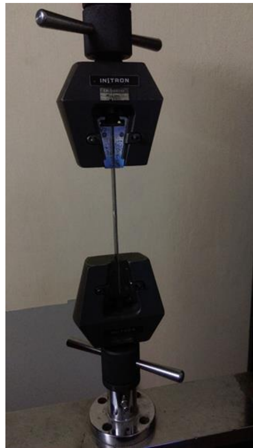
Figure 7: Tensile testing of a specimen
