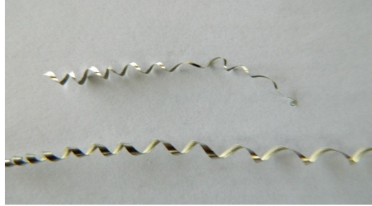
Figure 19. Intermediate shapes obtained during drilling
