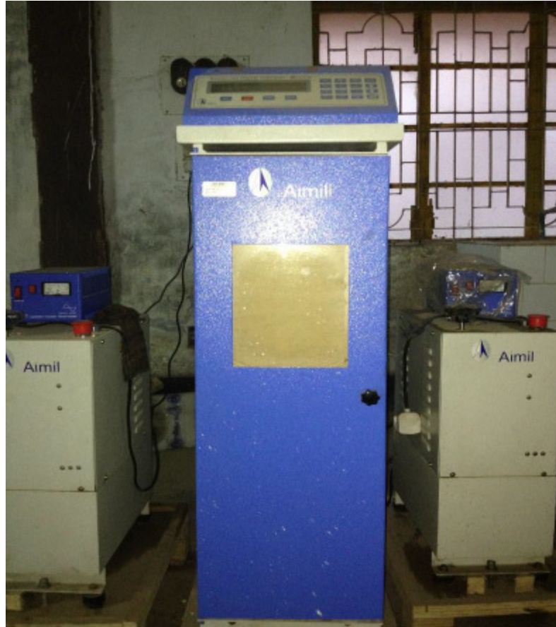
Fig 3.4 Testing machine for CCS measurement
