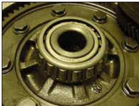
Figure 3.9: Tapered Roller Bearing - Manual Transmission`
