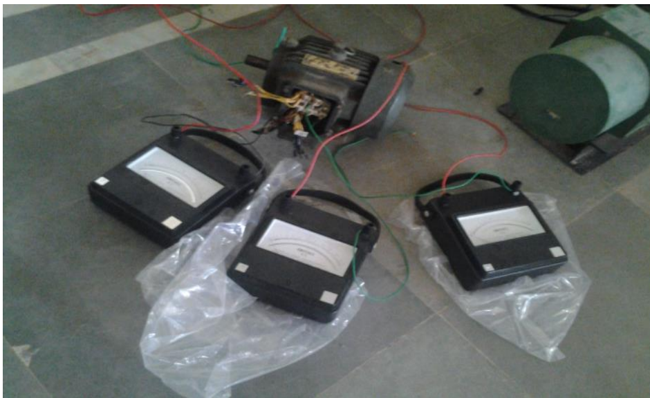
Fig.2.2 Experimental Setup of a 3 phase 2 hp Induction Motor connected to variac at no load
