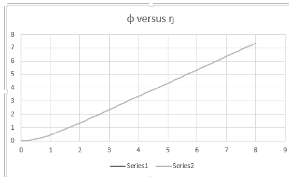
Fig. 3: Plot of \varphi versus \eta of the hiemenz flow
