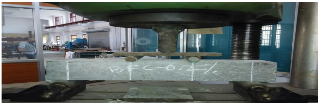
Fig. 3.5 Loading Arrangement for Load-Displacement Test
