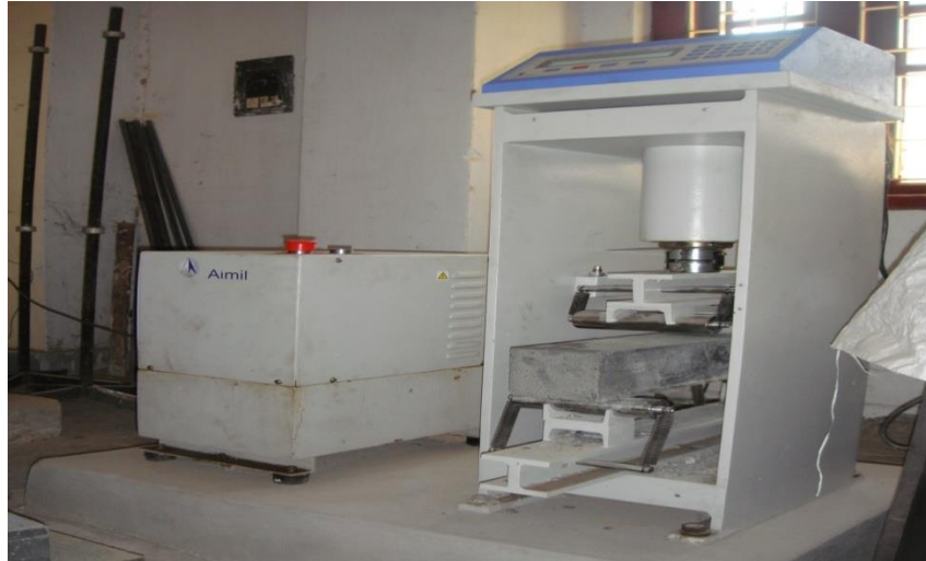
Fig.3.2.6.3 Flexure Test Set-Up
