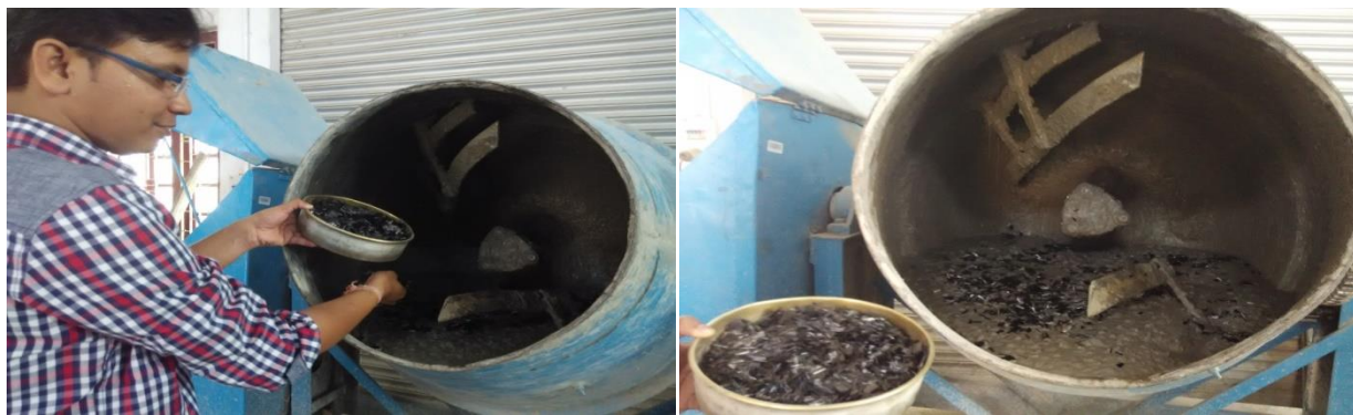
Fig. 3.3.1 Addition of Fiber to the SCC Mix
