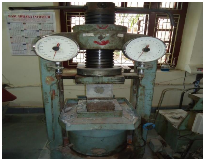
Fig: 3.2.6.1 Compression Test Set-Up
