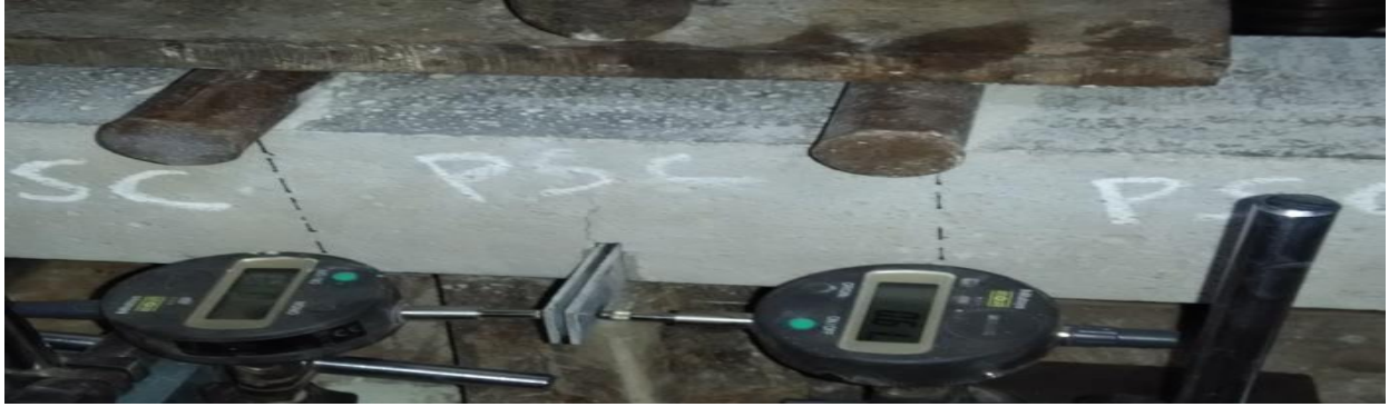
Fig 4.6.1 Crack Pattern of PSC
