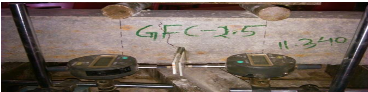
Fig.4.6.4 Crack Pattern of GFC-2.5
