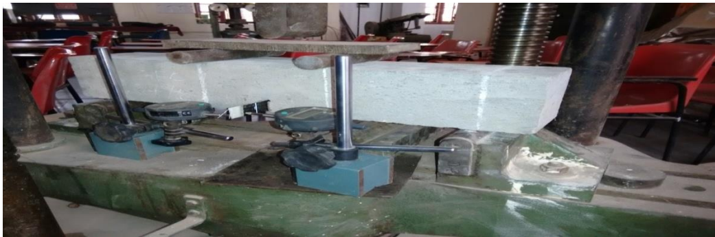
Fig. 3.5.2 Loading Arrangement for Fracture Test
