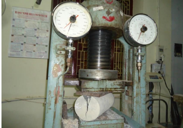
Fig: 3.2.6.2 Split tensile Test Set-Up
