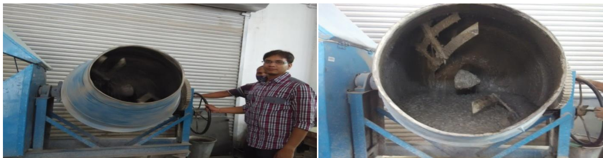
Fig.3.2.1 Concrete Mixture Machine & Preparation of SCC Mix
