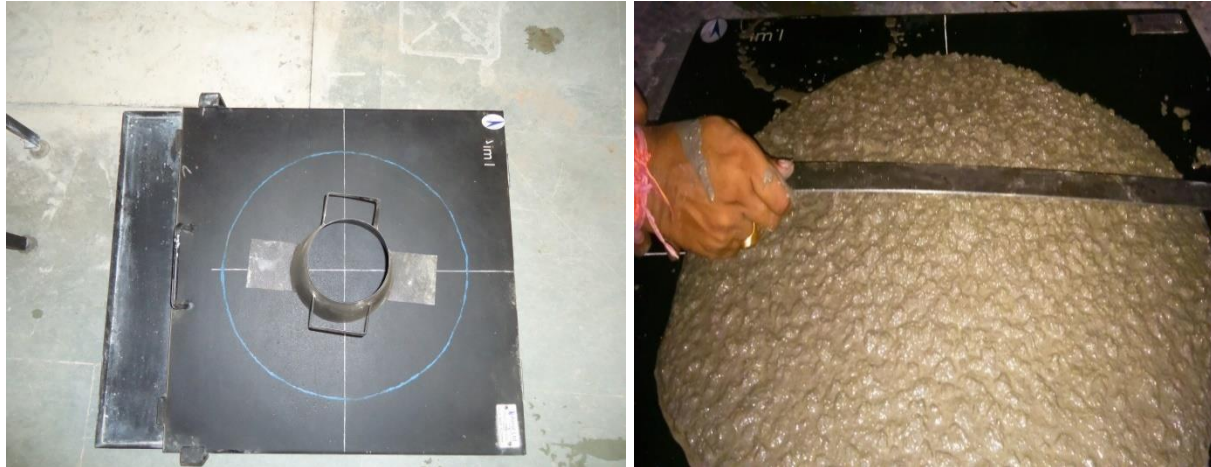
Fig. 3.2.3.1 Slump Flow Apparatus & Testing
