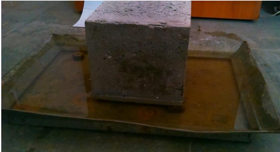
Fig. 3.7 Set-Up of Sorptivity
