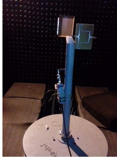
Fig. 5. 22 Far field measurement of the antenna array in anechoic chamber
