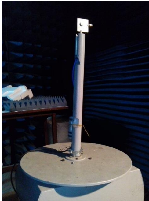
Fig. 5. 12 Far field measurement of the antenna element in anechoic chamber
