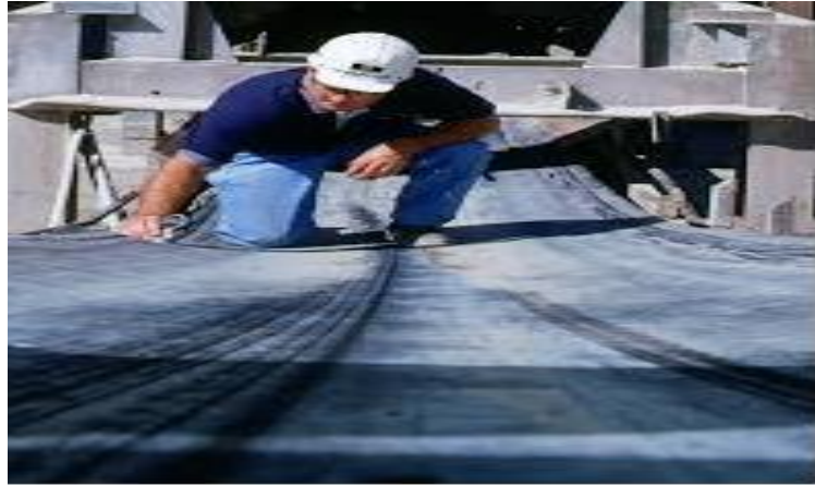
Visual detection by man on the surface of the conveyor belt.
