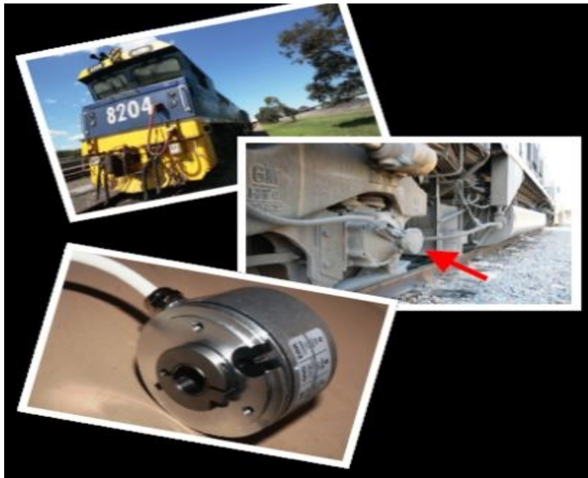
Monitoring the speed of diesel locomotive by sensor
