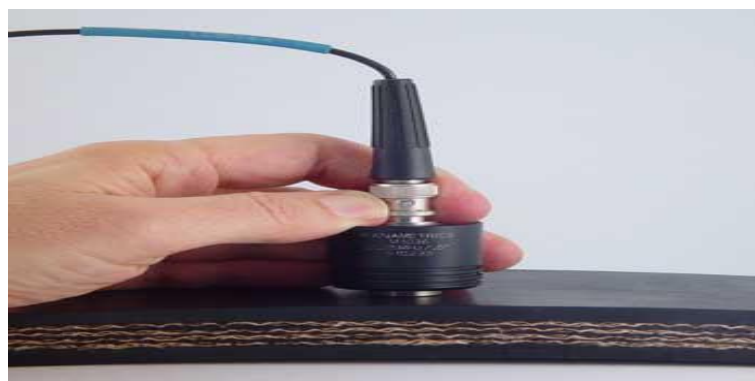
Thickness testing of conveyor belt
