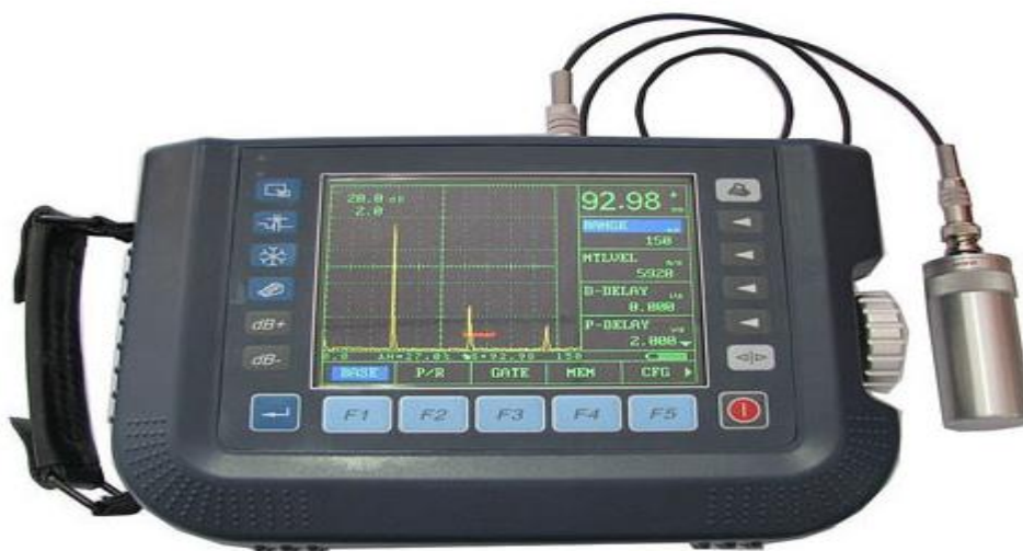
Minor crack monitoring by ultrasonic flow detector
