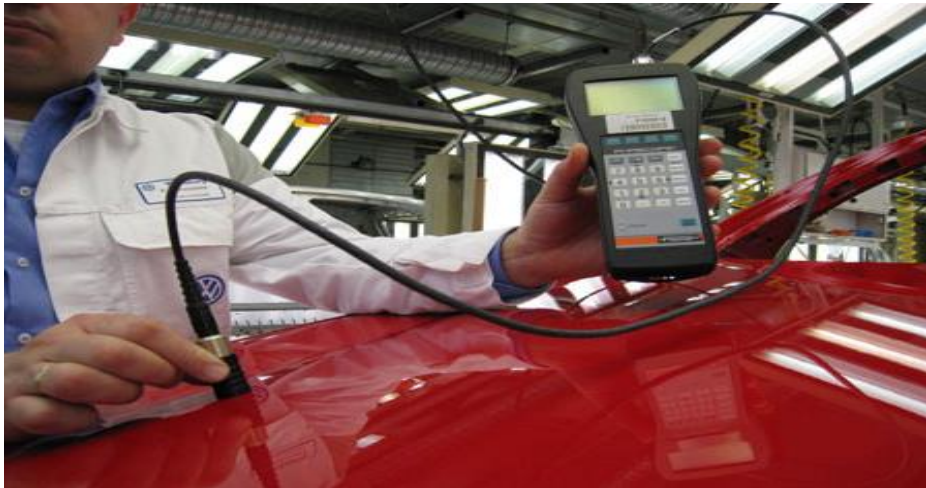
Ultrasonic thickness meter monitoring the thickness of paint and coating
