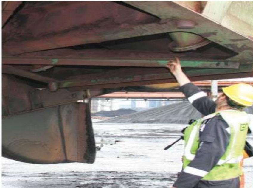
Stacker-reclaimer's distance from the stockpile monitoring by using Echomax XPS-30 ultrasonic transducer instruments
