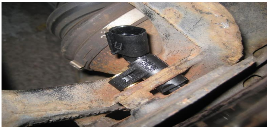
Wheel speed monitoring by sensor
