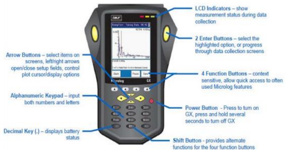
Vibration monitoring by Vibration analyser instrument
