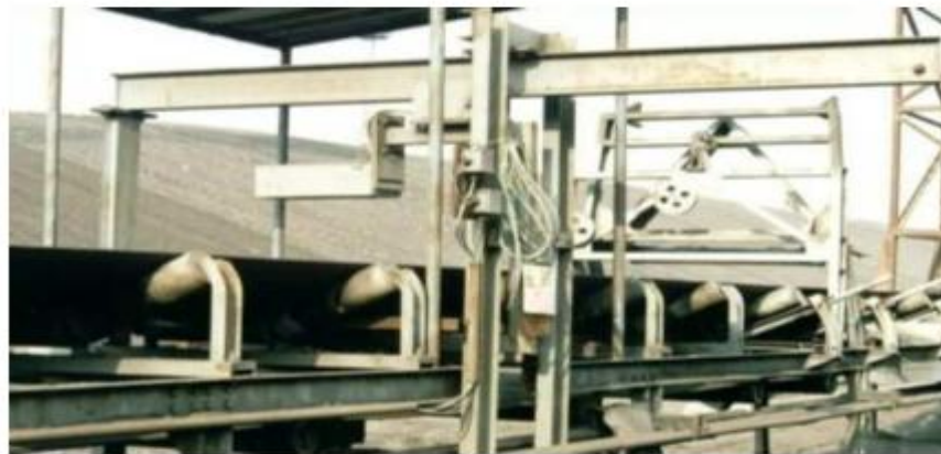
Online coal quality measurement by electric sensor
