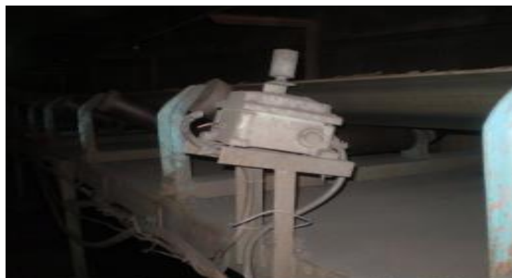
Belt sway switch is a protecting device for excessive running out and getting edge damaged
