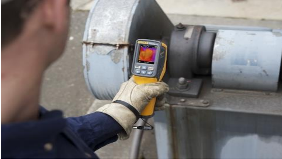
Hot spot detecting by infra-red thermometer
