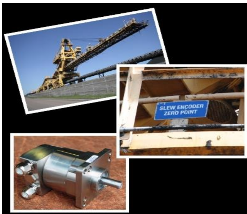
Stacker-Reclaimer position monitoring of luff, slew and long travel by using Hengstler AC61 series encoder
