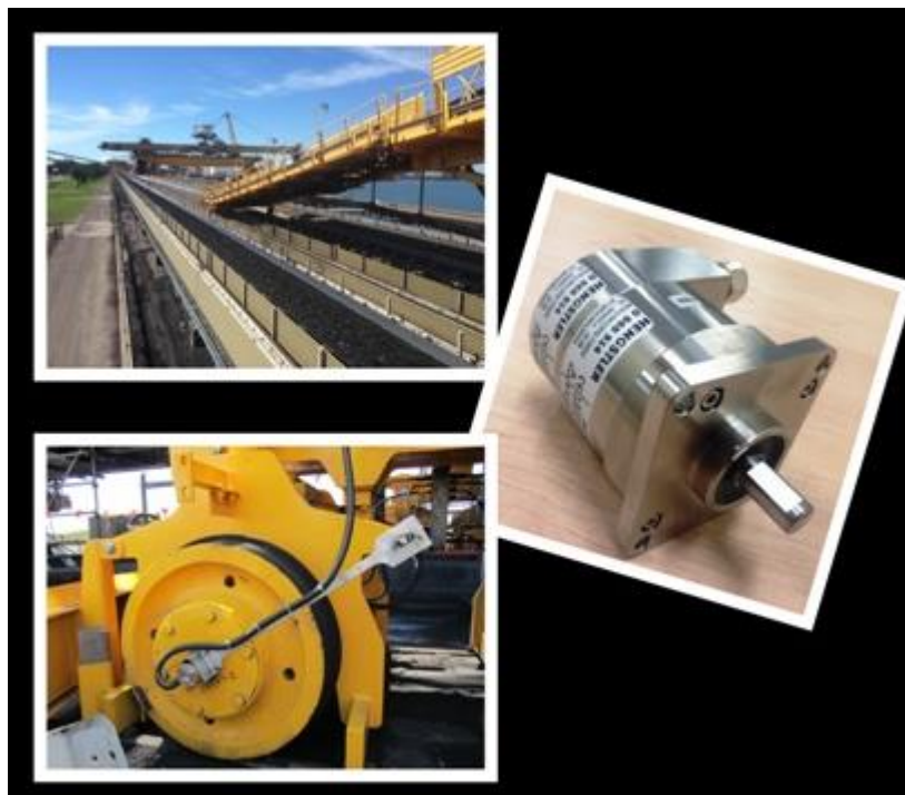
Machine long travel monitoring by sensor (Hengstler AC61 SSI multi-turn encoder)
