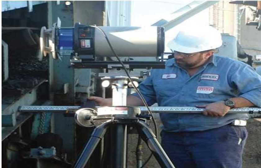
Laser Alignment is a highly accurate system to align framework and conveyor components
