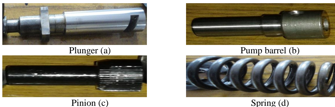
Fig. 6.74 Photographic view of the dismantled fuel injection pump components
