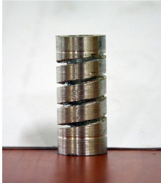
Fig 4.11: The machined spring
