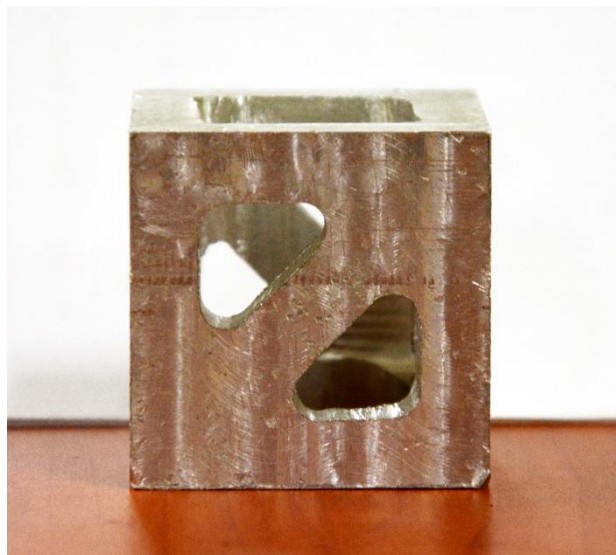
Fig 4.12: The force sensing structure
