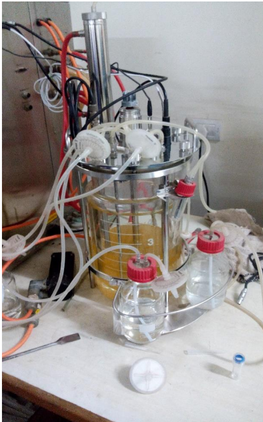
Figure 4. The setup of Bioreactor for fermentation of B.subtilis
