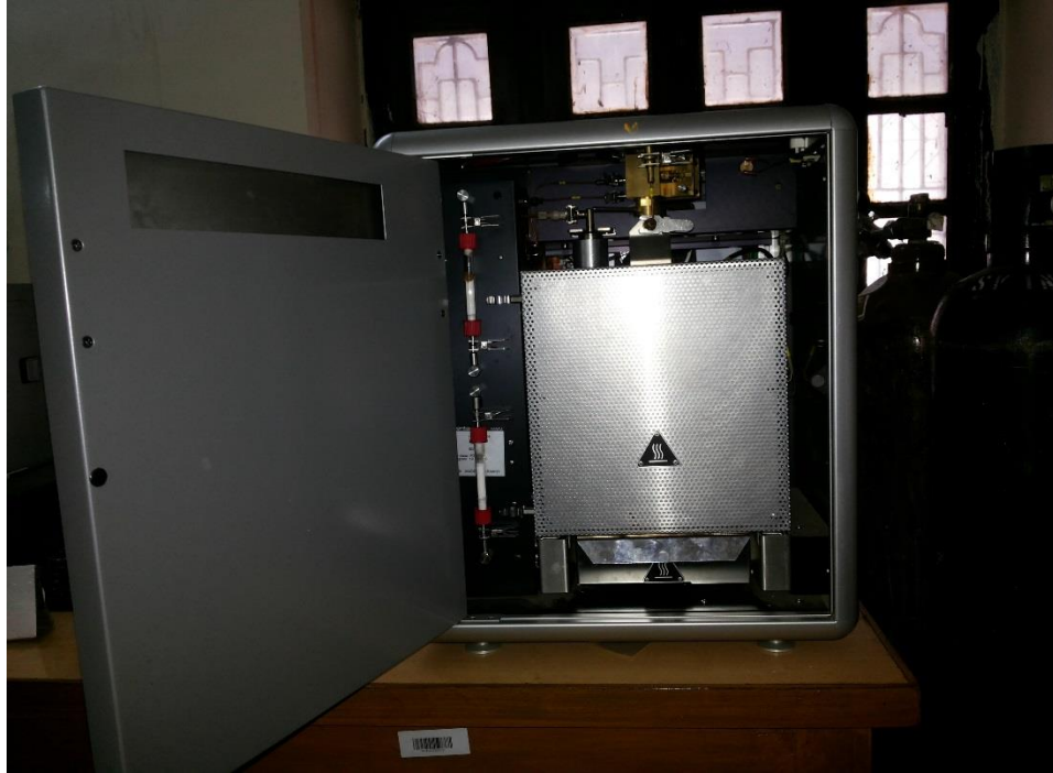
IMAGE 4(d): Carbon Hydrogen Nitrogen Sulphur ANALYSER (INSIDE VIEW)
