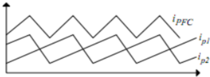
FIG 14(a): Input currents of two interleaved PFC circuits.
