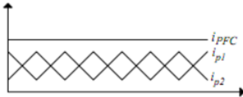
FIG 14(b): Input currents of two interleaved PFC circuits in ideal working condition.
