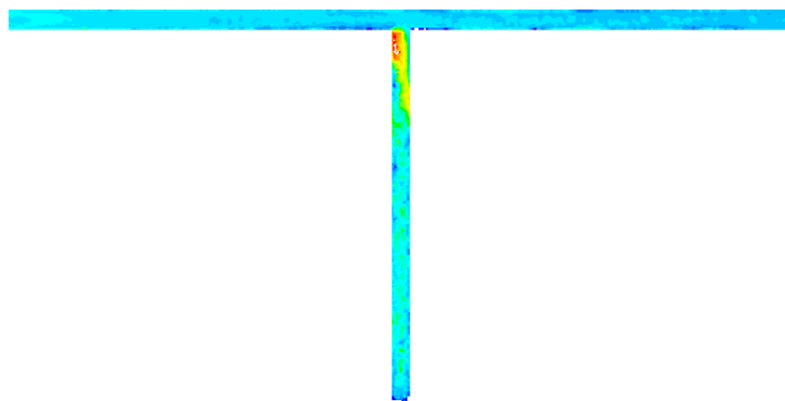
Figure 4.6: Phase contour at the horizontal midplane of the T-junction where, fluid pair is water-keresone, diameter is 0.05 m, velocity is 0.8 m/s & volume fraction is 0.4.
