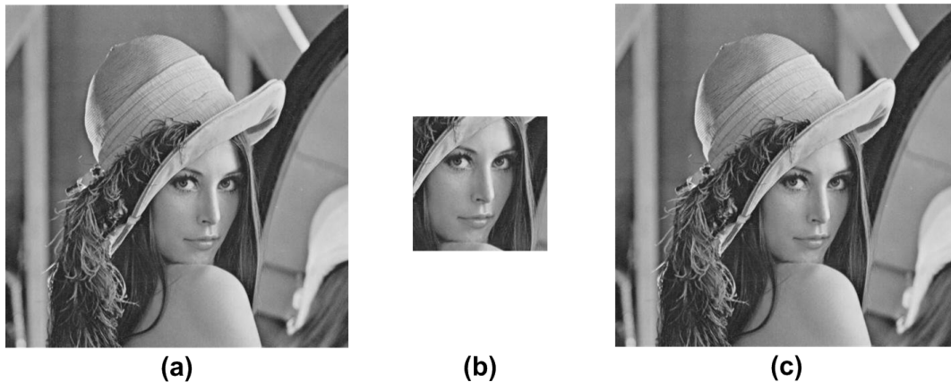
Figure 3.1: Lena JPEG images: (a) Original Lena 512 \times 512 image; (b) Central 200 \times 200 portion/region which is re-saved at a different degree of compression; (c) Forged Lena image in which the central portion/region is modified.
