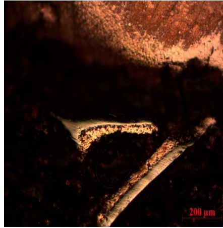
Figure 4.2. Optical micrograph of the cross-section of a Cu-Ni multilayer composite, heated at 900°C for 1 hr
