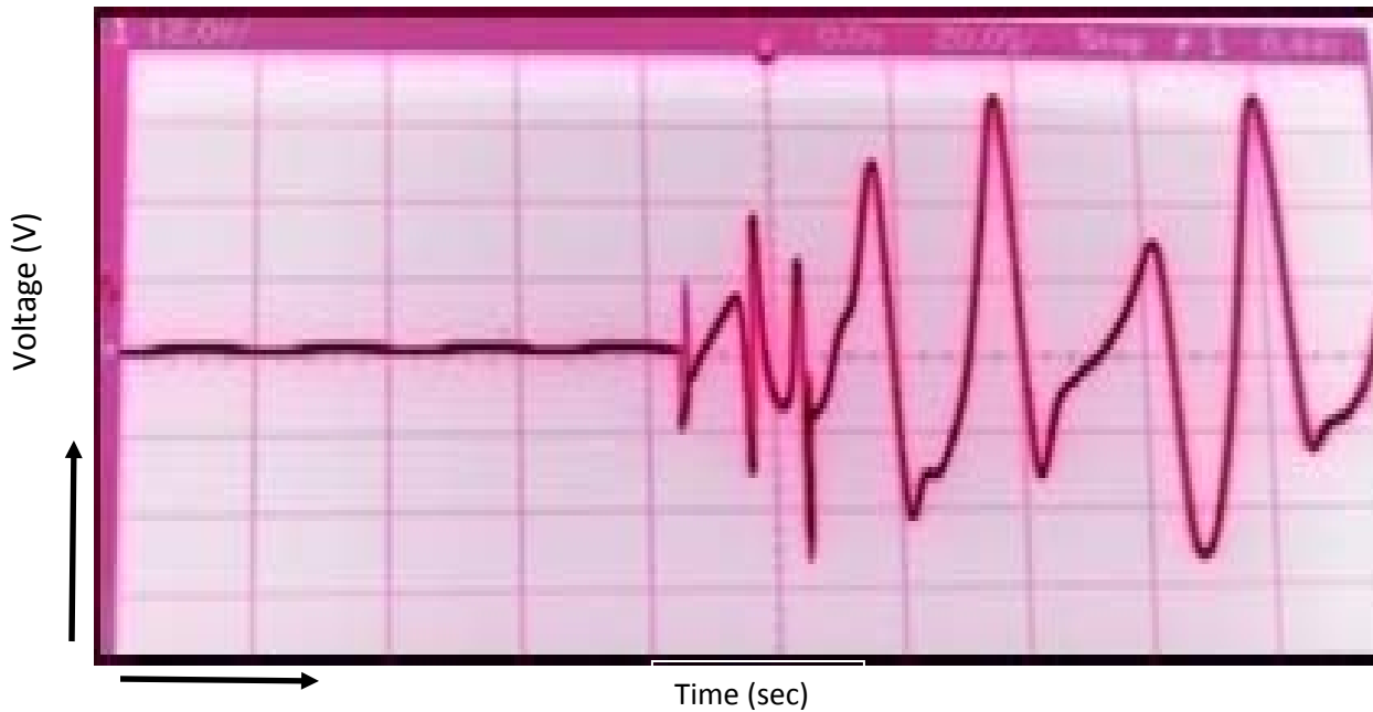
Fig.5.9 Stator voltage waveform during the voltage build-up for a prime mover speed of 1440 r.p.m.
