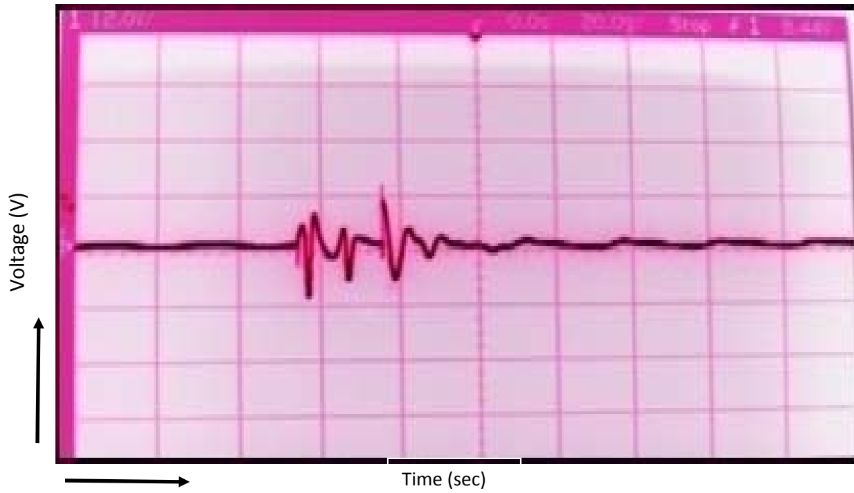
Fig.5.12 Waveform showing failure of build-up for a prime mover speed of 1090 r.p.m.
