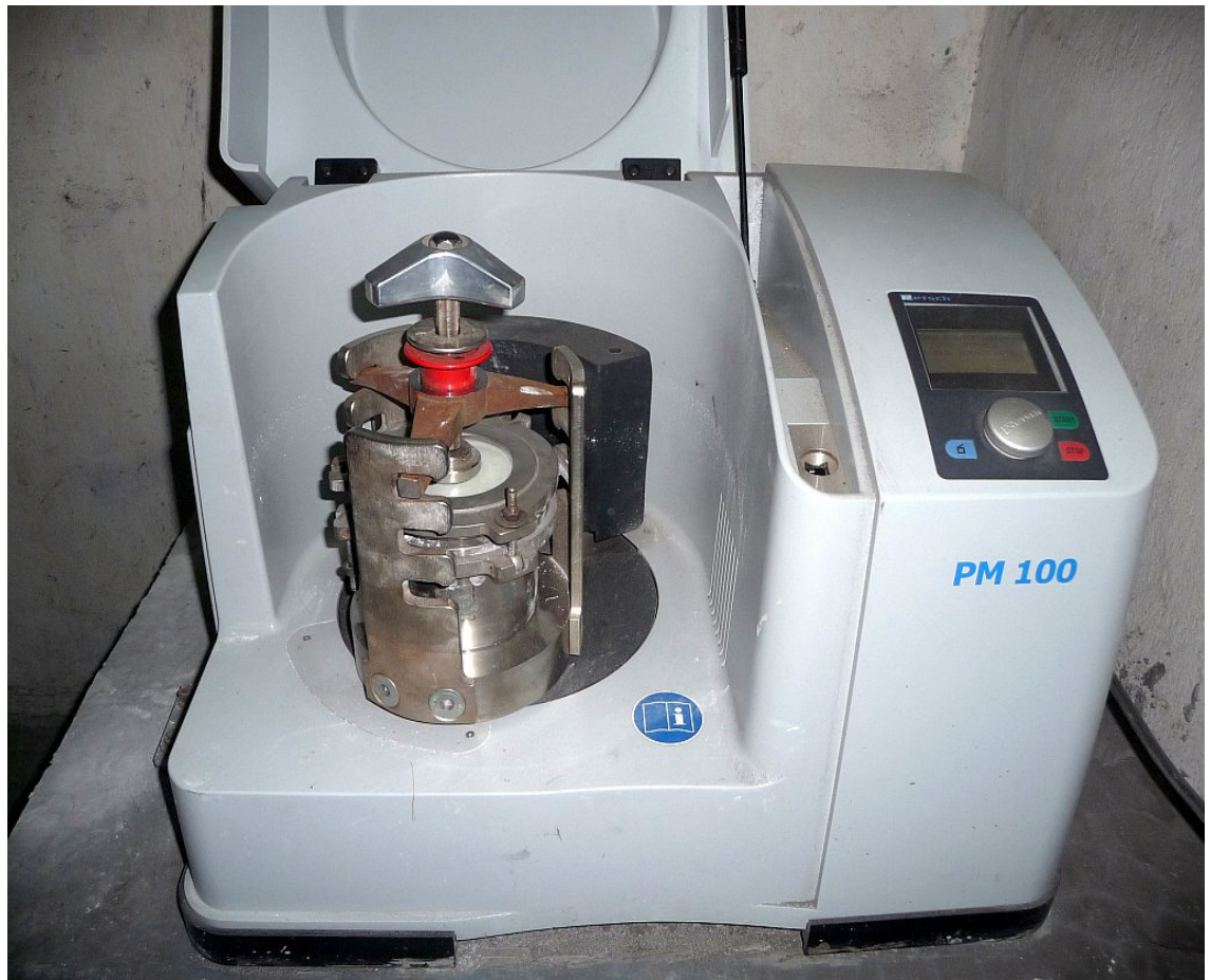
Photograph 3 Planetary ball mill (Para 2.9.1)
