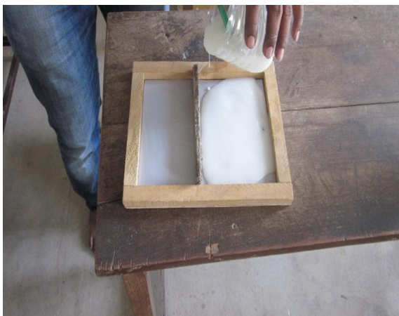
Fig 4.14 Particulate filled epoxy composite fabrication by hand lay-up process
