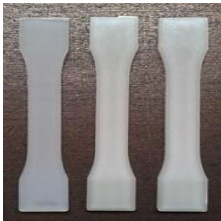
Figure 4.21 Composite samples for tensile test and its loading arrangement
