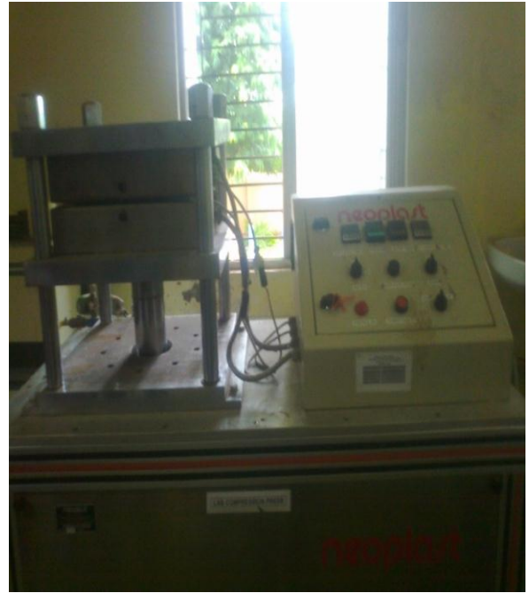
Fig 4.15 Haake Rheomix 600 batch mixer Fig 4.16 Compression moulding machine
