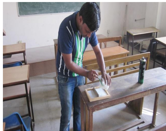
Fig 4.14 Particulate filled epoxy composite fabrication by hand lay-up process
