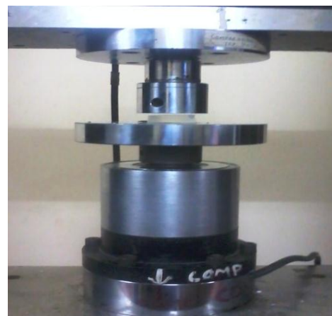
Figure 4.22 Composite samples for compression test and its loading arrangement
