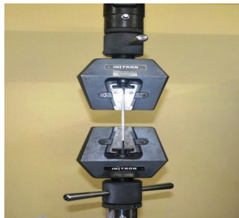
Figure 4.21 Composite samples for tensile test and its loading arrangement
