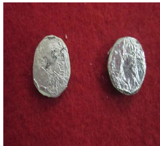
Fig 4.26 Aluminium foil wrapped test samples for dielectric test
