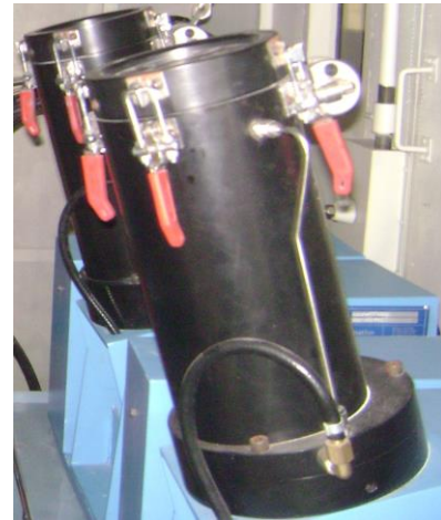
Figure 3.8 Mixing chamber in which premixing of \text{Al}_2\text{O}_3/\text{TiO}_2 with LD slag is done
