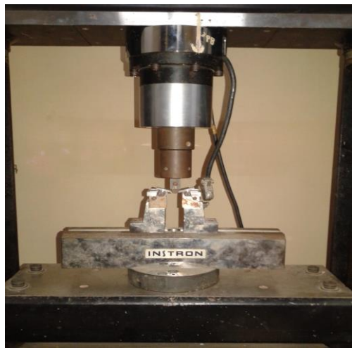
Figure 3.23 (b) Loading arrangement for flexural test
