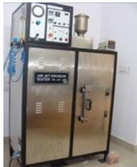
Figure 3.24 (b) Solid particle erosion test set-up
