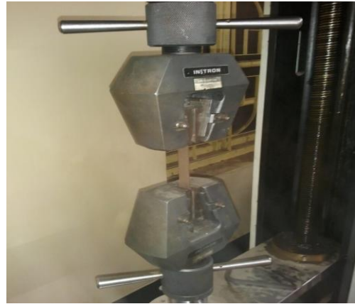
Figure 3.22 (b) Loading arrangement for tensile test
