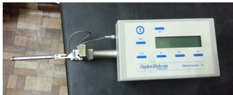
Figure 2.16 Talysurf (Model: Taylor Hobson, Surtronic 3+)
