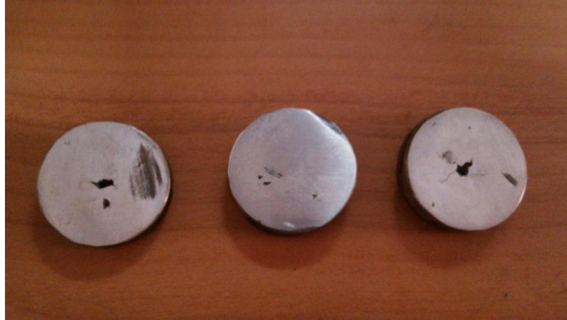
Figure 2.27 Three samples of workpiece at three different feed rates
