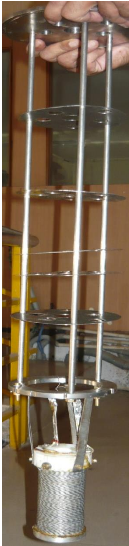
Fig 4.5 (Left) Magnet with support structure (Right) Cryostat Flange
