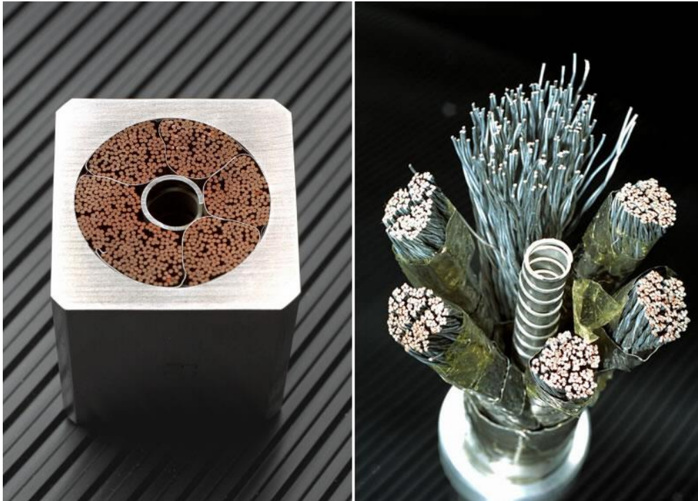
Fig 1.17: Section of the CICC conductor [33]
