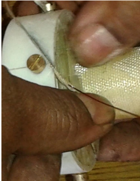
Fig 2.7 Nb-Ti superconducting wire is being passed through sleeves in cut slot.
