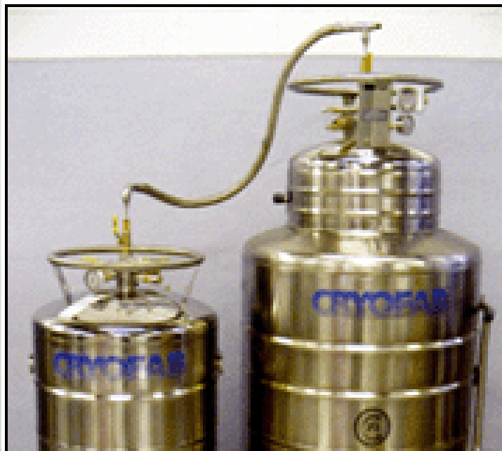
Fig 4.4 Helium Transfer from plant dewar to test dewar
