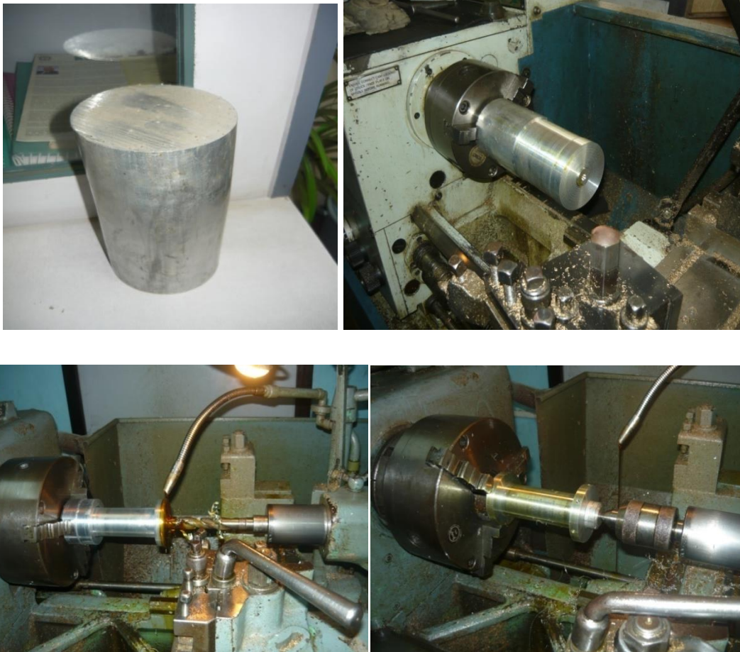
Fig 2.2: Various stages of former making (a) starting aluminum rod (b) machining of rod in lathe machine (c) boring of central hole (d) finalizing the former.
