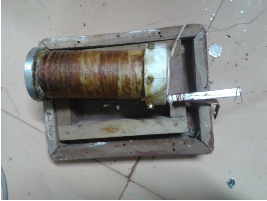
Fig 2.12 Fibre glass cloth wrapped superconducting magnet left for drying
