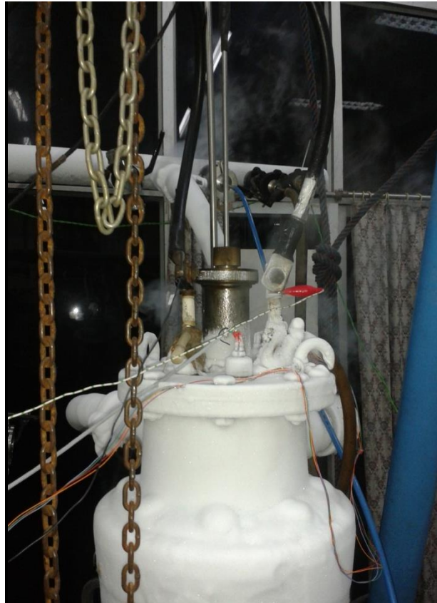
Fig 3.7 Frosting over the cryostat, while transferring liquid helium to the cryostat
