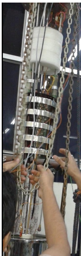
Fig 3.5 Magnet being inserted inside the cryostat, with the help of chain and pulley arrangement.
