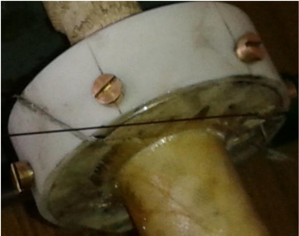
Fig 2.6 (top) Slot cut is being made, to take the superconducting wire out. (Below) Complete mandrel with slot
