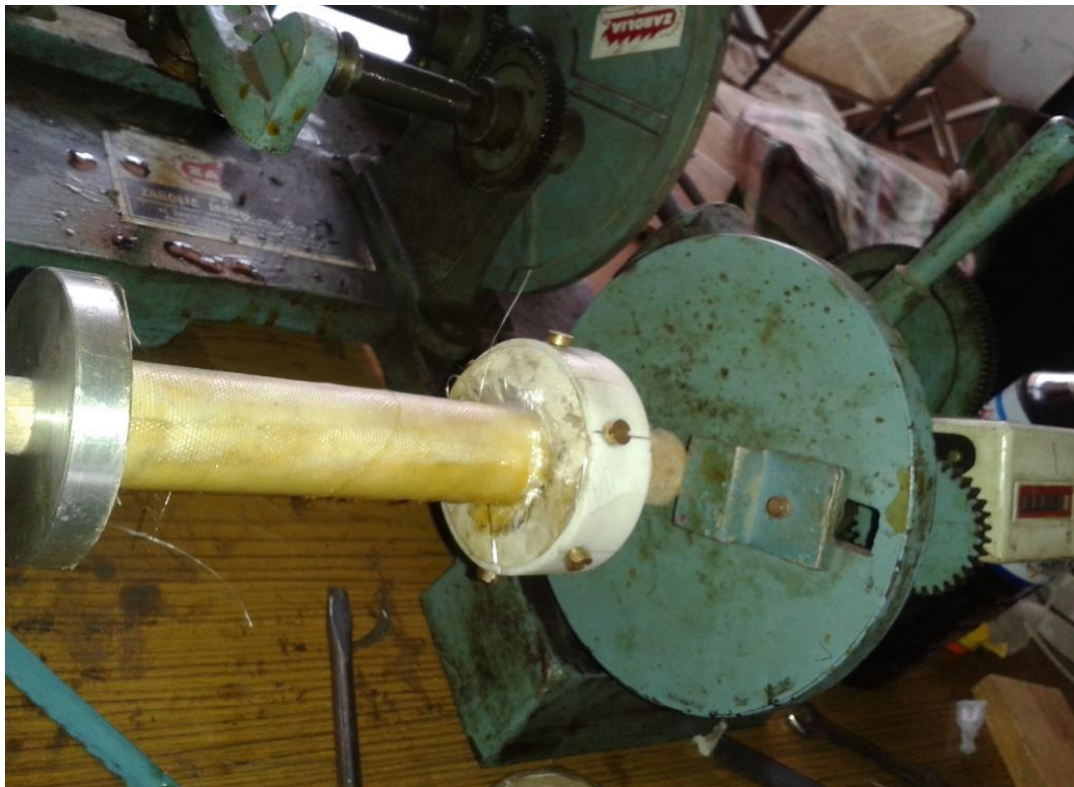
Fig 2.4: Fibre glass cloth being wound on the mandrel for insulation and for providing winding base
