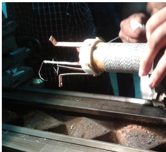
Fig 2.13 Racquet thread being wound on top of the fibre glass cloth wrapping.
