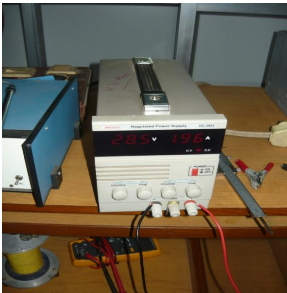
Fig 2.5 Testing of copper wire magnet for magnetic field generation. (Top) At room temperature, 0.26 A current is passed to get 50G magnetic field. (bottom) At 77K, the current could be raised to 1.96A.
