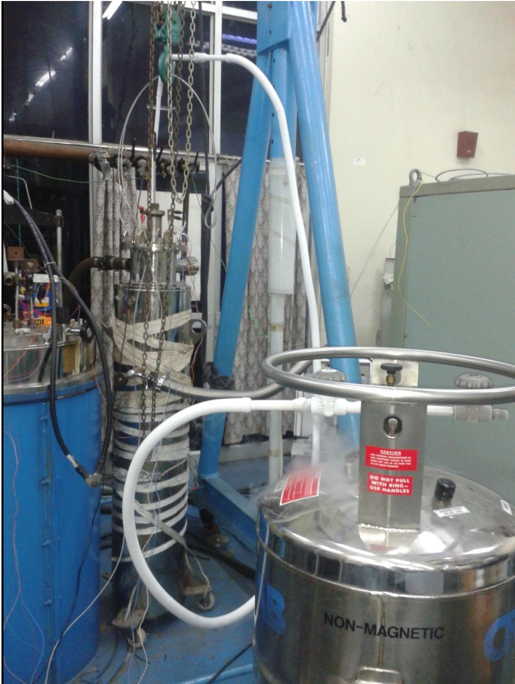
Fig 3.6 Pre-cooling of cryostat using liquid nitrogen
