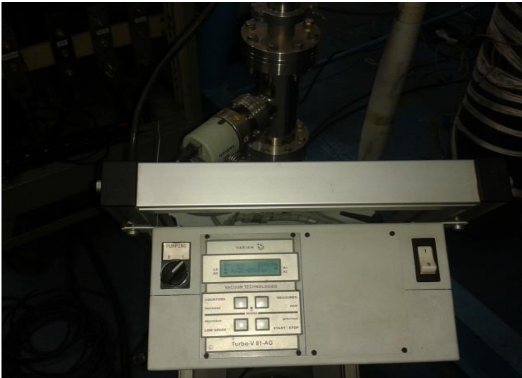
Fig 3.2 (top) Evacuation of cryostat with backing, by turbo molecular pump (bottom) front of vacuum pump
