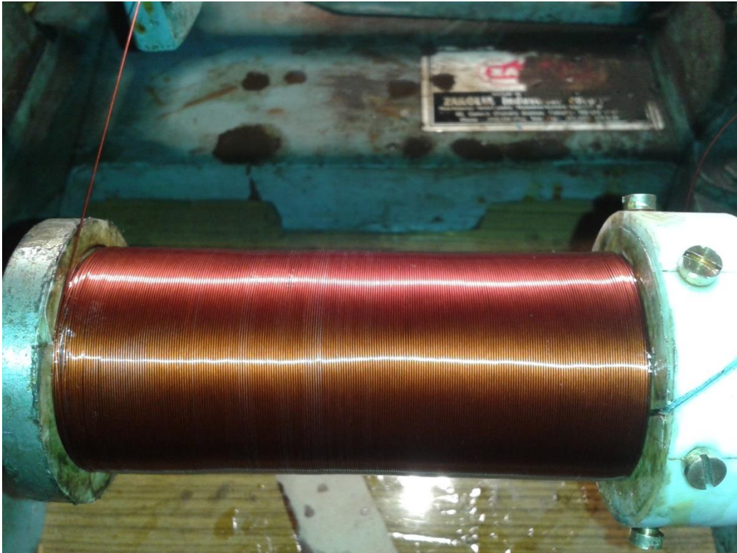
Fig 2.10 Final layer of superconducting winding, without fibre glass cloth
