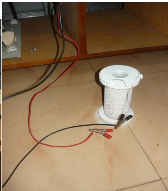
Fig 2.5 Testing of copper wire magnet for magnetic field generation. (Top) At room temperature, 0.26 A current is passed to get 50G magnetic field. (bottom) At 77K, the current could be raised to 1.96A.
