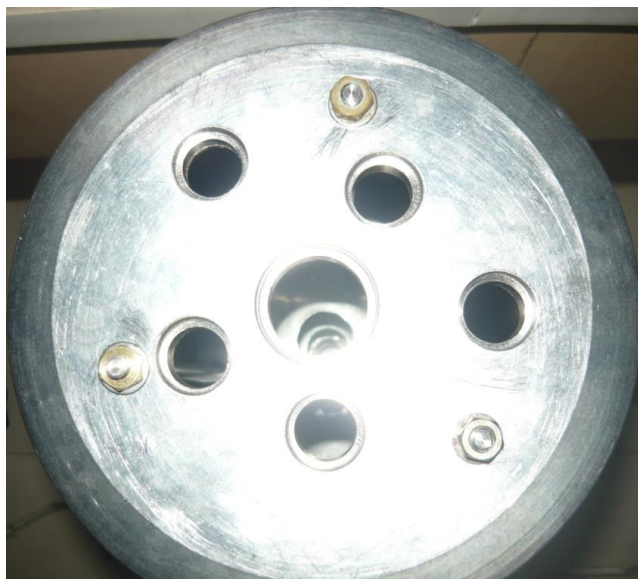
Fig 4.5 (Left) Magnet with support structure (Right) Cryostat Flange
