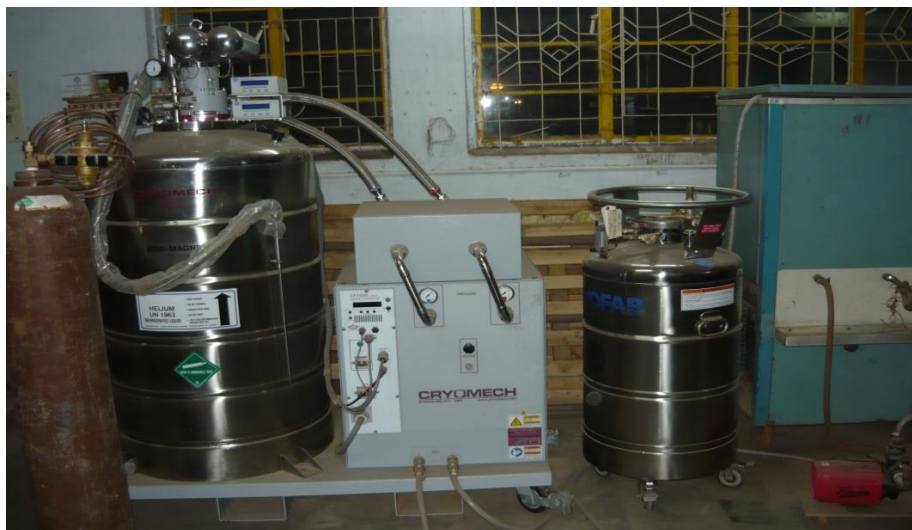
Fig 4.6 LHe Test facility for superconducting magnet testing
