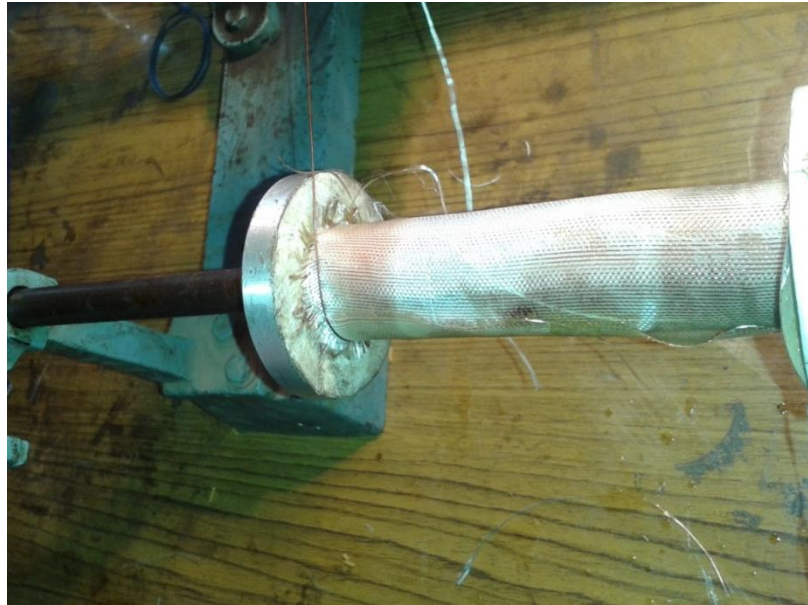
Fig 2.8 Fibre glass cloth wound over the intermediate layers.
