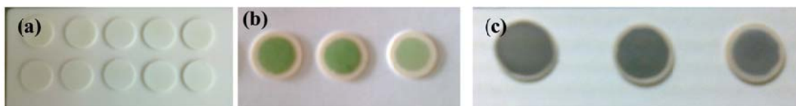
Fig. 3.2: Photograph of dense YSZ (a), symmetrical cells before (b) and after (c) reduction.
