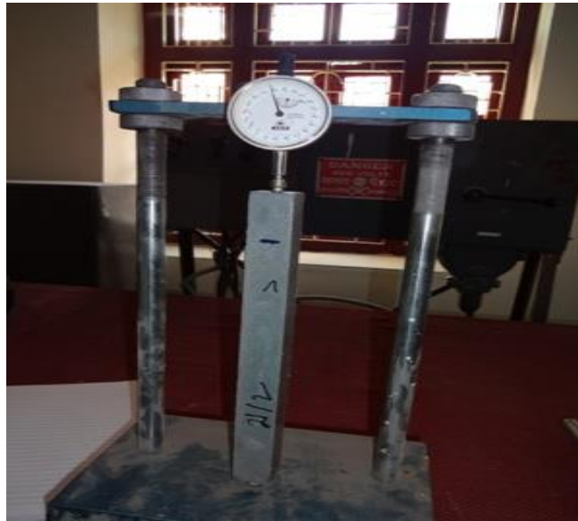
Figure 3.2 Length comparator with beam mould
