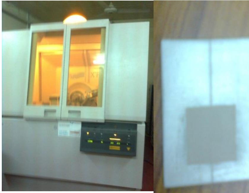
Figure 3.6 Philips X' PERT System X-Ray Diffractometer with sample holder
