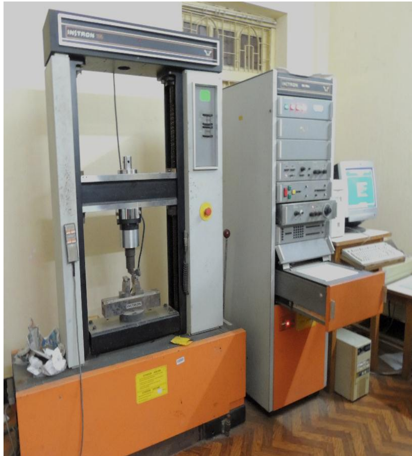
Figure 3.1 Universal testing machine, Instron 1195
