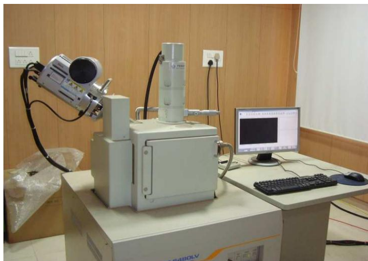
Figure 3.5 Scanning electron microscope setup
