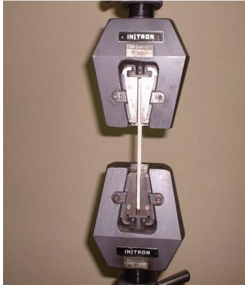
Figure 3.2 Loading arrangement for tensile test
