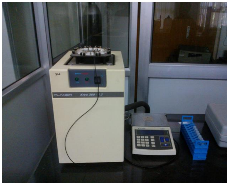
Figure 3: Controlled rate freezer for cryopreservation of MSCs
