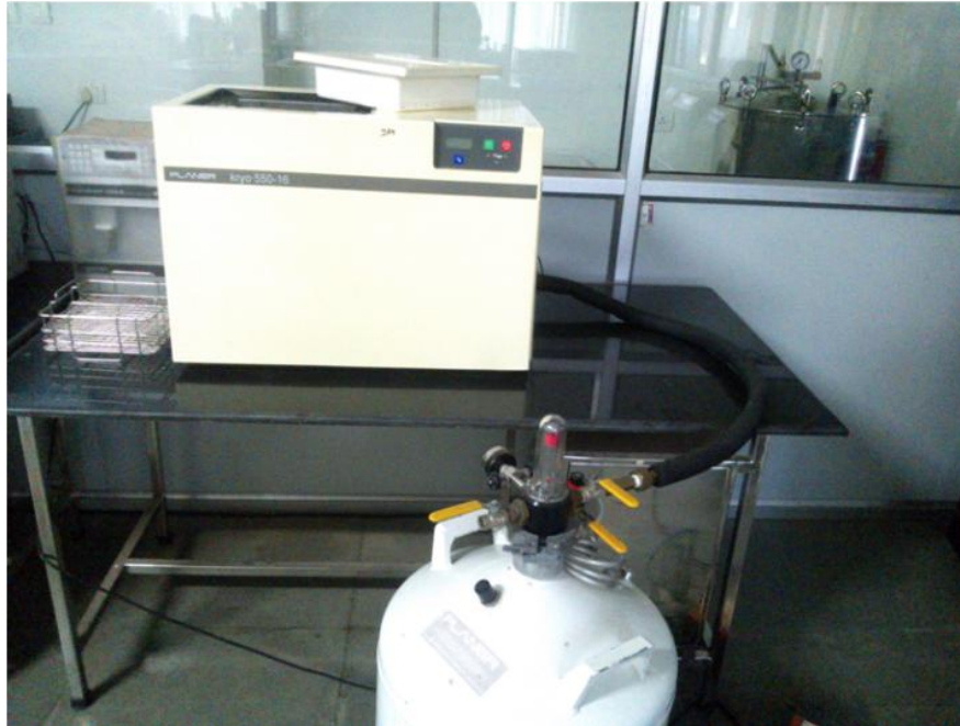
Figure 4: Controlled rate freezer for cryopreservation of TECs
